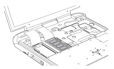
Figure 8-12 Raising the insulation sheet
